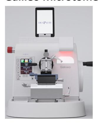
Ultra-smooth-running handwheel with exclusive electronic locking system in each position equipped with ergonomics and retractable handle. Backlit panel for an immediate sample detection Spaciously designed section waste tray with fixing system. Roomy shelf equipped with removable tray. Emergency stop push button Galileo Series 2
