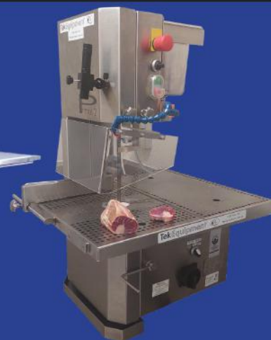
Primus 2 - Benchtop • 50 x 59 x 87cm external dimensions • 40cm working height • 21cm cutting height
