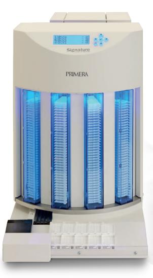
Creates 2D Barcodes for Specimen Tracking
